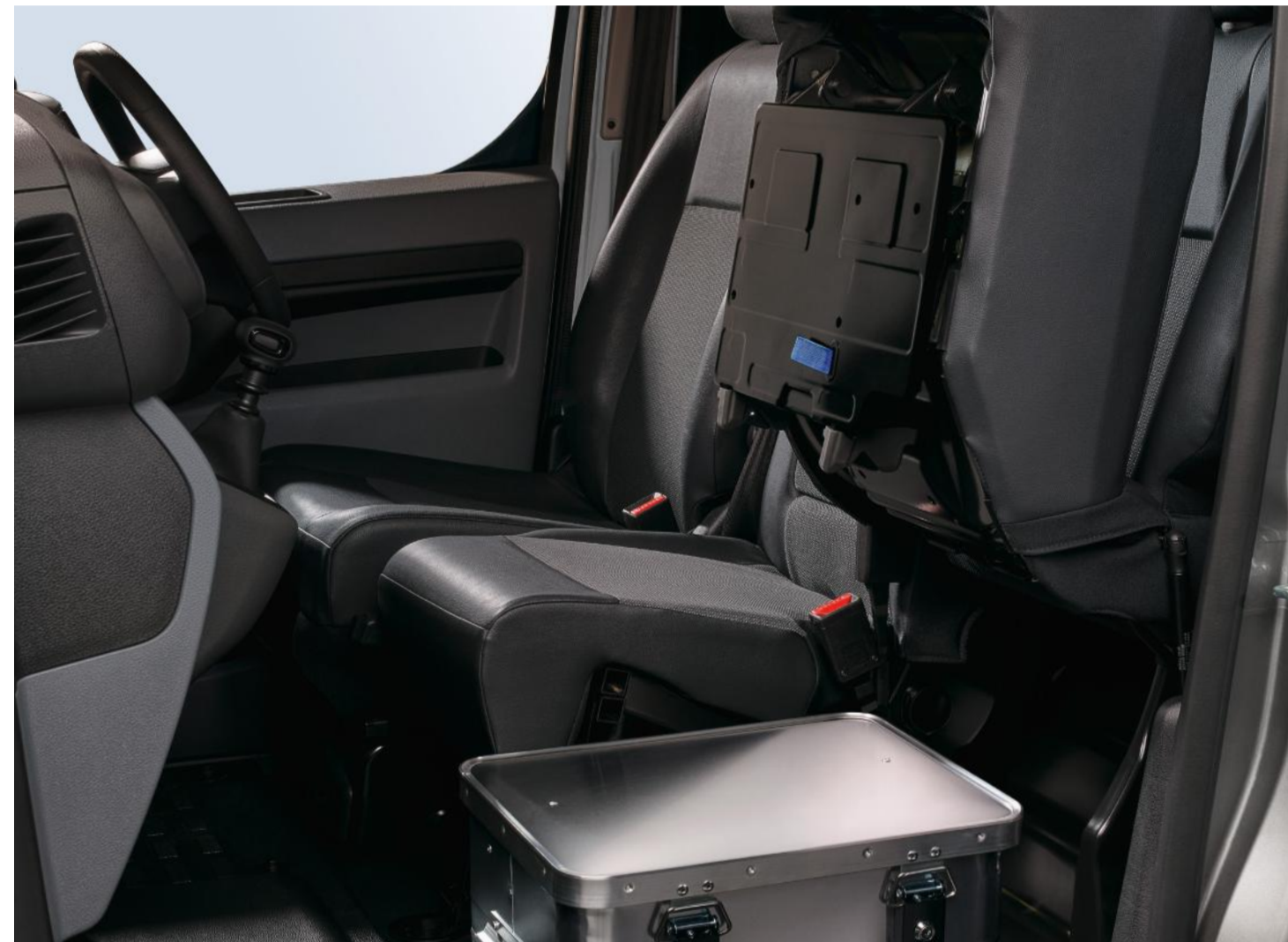
Load-through hatch within bulkhead.
