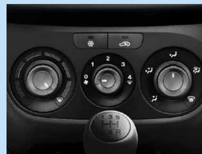
Air conditioning and air recirculation.
