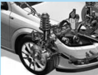
MacPherson strut front suspension.
