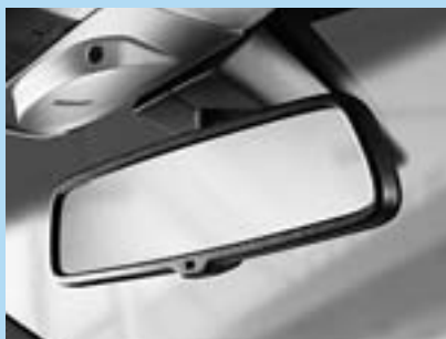
Electro-chromatic anti-dazzle rear-view mirror.
