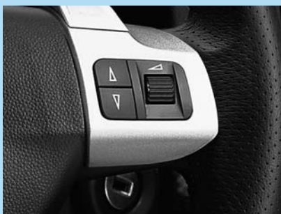
Steering wheel mounted audio controls.
