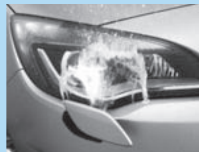
High-pressure headlight washers.
