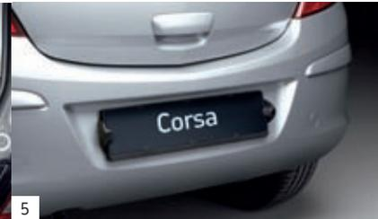
**Rear parking distance sensors.** [5] Activated automatically as you select reverse, this clever system beeps faster the closer you get to an obstruction, changing to a continuous tone at 30cm away.
