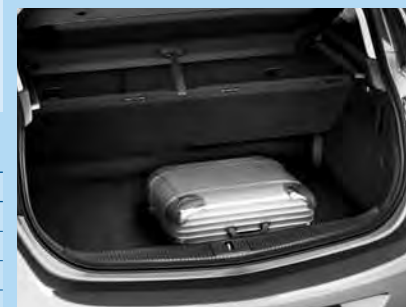
Flex Floor – adjustable luggage compartment floor – Hatchback.
