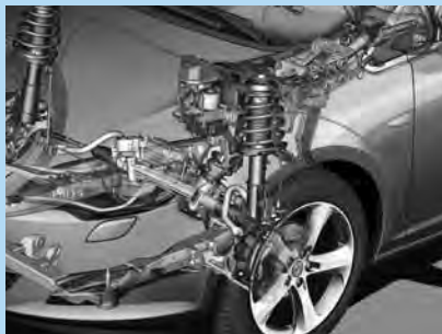
MacPherson strut front suspension.
