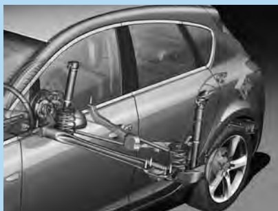
Compound crank rear suspension includes innovative use of Watt's link
