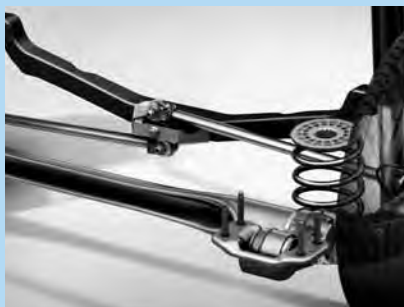
Watt's link improves handling and ride comfort.
